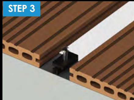
STEP 3 Position Fixing Clip into rebate at the side of the board and screw tight (6mm or 10mm)
