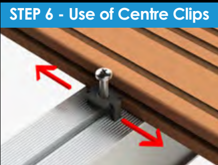
STEP 6 - Use of Centre Clips The Centre Clip is important for installs in extreme climates and where shading occurs and expansion gap consistency is aesthetically important.
